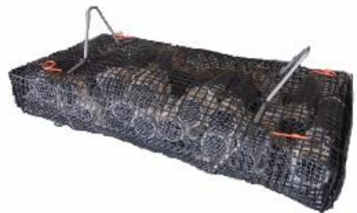
Figure 2b: re-immersion bag containing 25 plastic tubes
