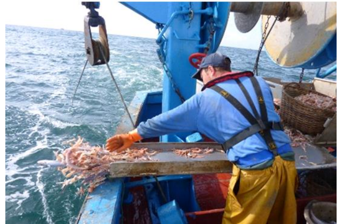
Figure 6 : sorting gutter to discard the con-commercial catch all along the sorting process on board
